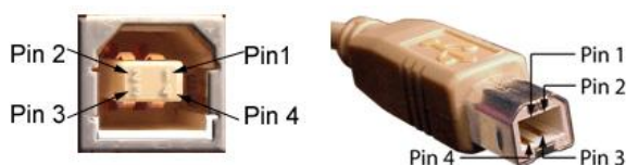
Figure 23 Pinout of USB Console interface
